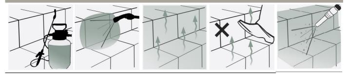
STEP 1. Fill a light pressure sprayer with the solution. Do not dilute. STEP 2. Set the pressure between 0.5 and 1 bar. Apply an even layer to the surface. STEP 3. Leave the solution to penetrate the surface. Leave for 1 – 5 hours depending on the level of soiling. STEP 4. Keep off of surfaces, while the solution is active. Keep pets and children away STEP 5. Rinse well with plenty of water. Allow surfaces to dry before allowing traffic or sealing applying porcelain protector.
