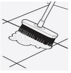
STEP 3. Grout in the joints or brush in jointing compound and clean off residues. Always follow manufacturers instructions.
