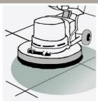
STEP 3. Scrub surfaces with a rotary scrubber to release cement & salt residues.
