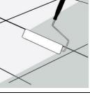
STEP 2. Spread out evenly using a sealant applicator pad, broad paint brush or foam roller. Repeat after 30 minutes. Leave to dry for 1 hour.
